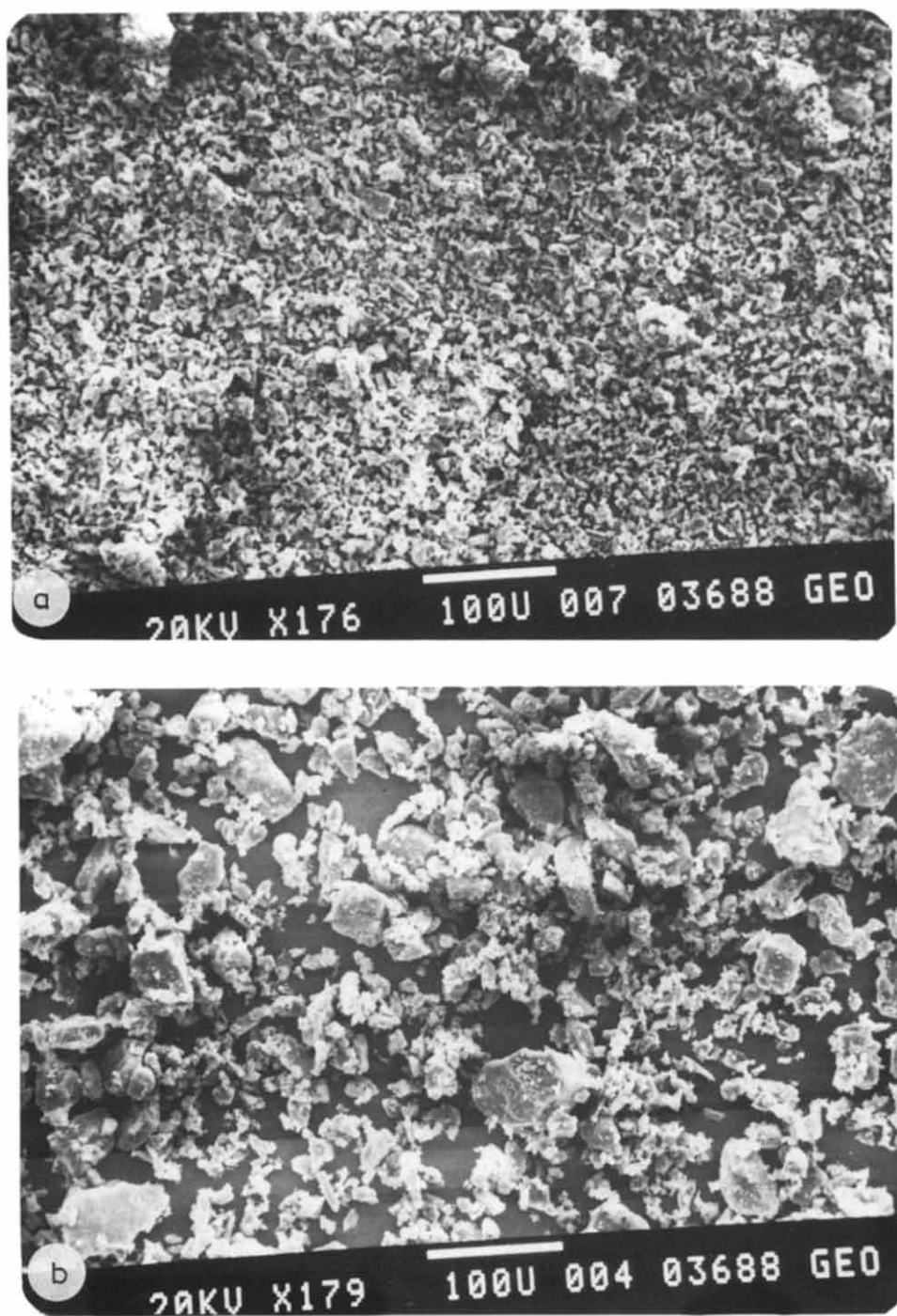
Fig. 2. ESM photomicrographs of calcium hydrogen phosphate (a, \times 176 ), lactose (b, \times 179 ), sucrose (c, \times 172 ) and maize starch (d, \times 1720 ).
